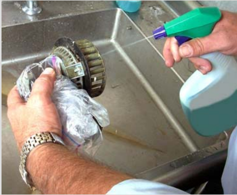
Cleaning the blower motor ensures even combustion.
