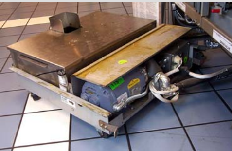
Heater tapes should be checked.
